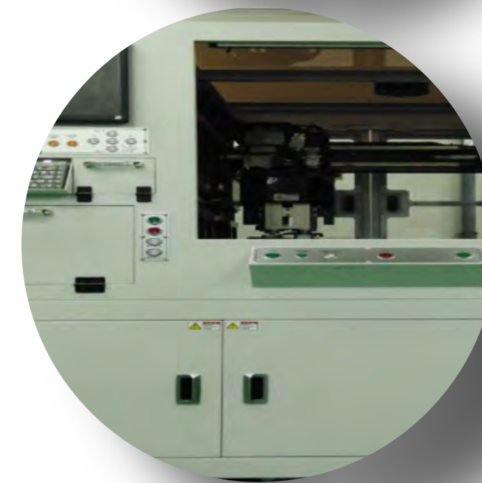
Auto stiffener placement
