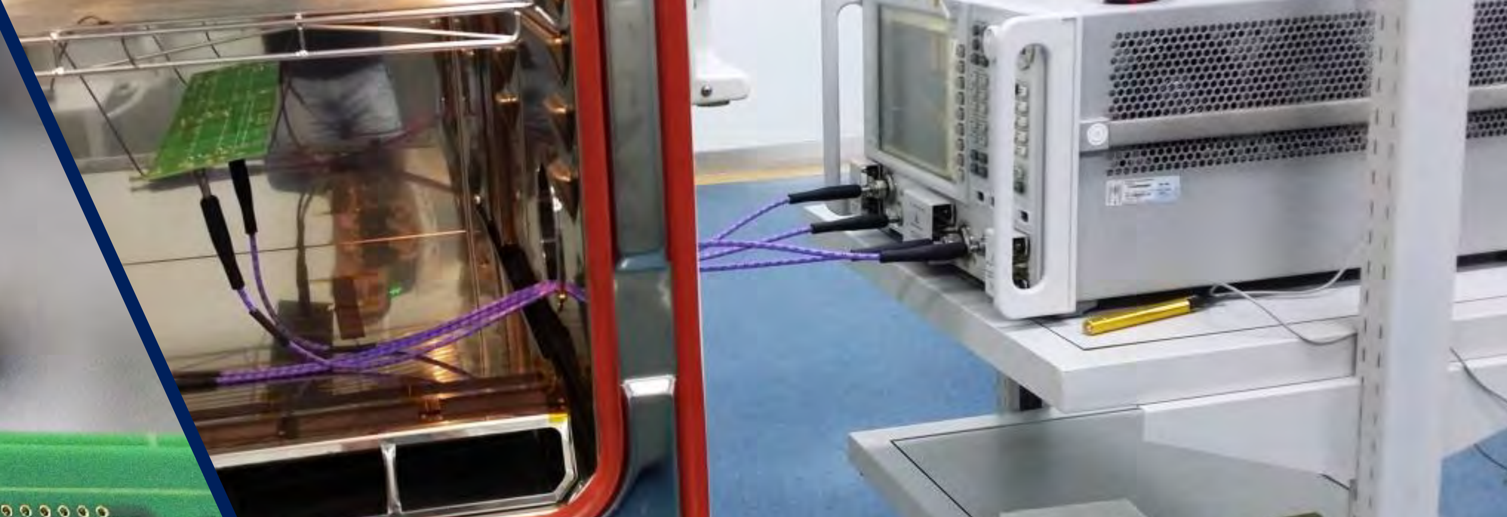
Capability to measure effects of ambient environmental temperature and humidity on signal integrity
